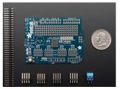
Adafruit 16-channel PWM/Servo Shield 16 channels of servo-bustin' power
