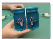
Modifying Servos for Continuous Rotation Make tiny gear-motors for your next robot!
