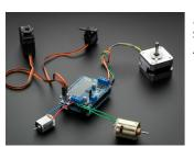
Adafruit Motor Shield V2 for Arduino Stackable, high current DC and Stepper motor shield for Arduino
