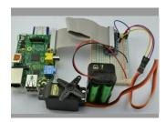
Adafruit's Raspberry Pi Lesson 8. Using a Servo Motor Write a Python program to control a servo motor with a Raspberry Pi
